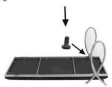
Assemble the one of body panel and tighten the screws with the cushion.
