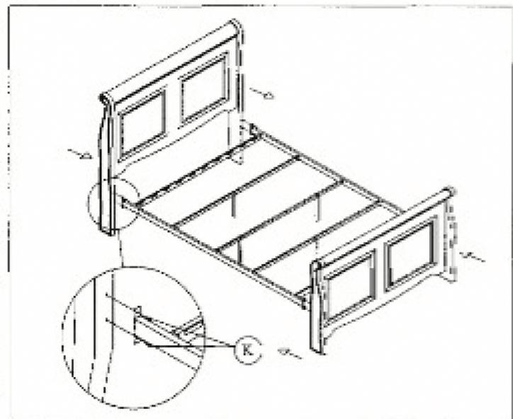
**Step 5** Assemble bed base into bed frame and tighten all bolts.
