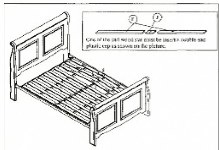
**Step 6** Once wood slats have been inserted into the plastic caps, fix one end of wood slat into the hole of end cross bar G and the other end to the other end cross bar. After that fix the plastic cap to the center cross bar by pressing it accordingly to the default holes. Ensure the plastic caps put aimed to the hole.
