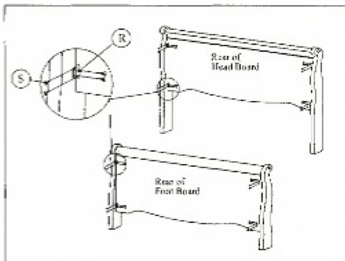
**Step 2** Fix horizontal bracket at headboard & footboard as shown.
