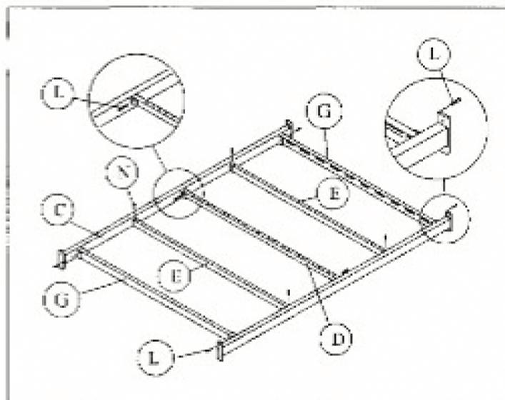
**Step 3** Fix both side rails and cross bar D with bolt L, as shown diagram. Put cross bar E into side rail and fix it with bolt N. After that put end cross bar G to the end of side rail and tighten with bolt L.
